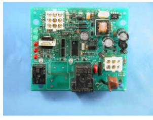
Original NM and FM Controller Production: 1988-1990 Service: No longer available, replaced by AutoSentry kit. Had reset switch
